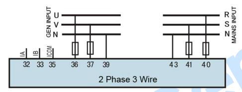
Fig.7 2-Phase 3-Wire Connection Diagram
