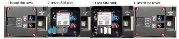
Fig.9 SIM Installation Steps
