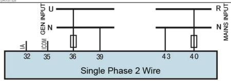
Fig.6 Single Phase 2-Wire Connection Diagram
